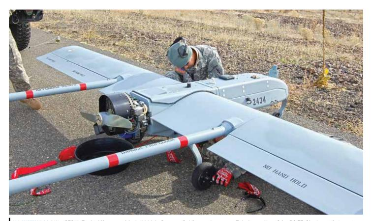
ALL SYSTEMS GO A 1st SFG(A) Tactical Unmanned Aerial Vehicle Systems Soldier conducts a preflight inspection of the RQ-7B Shadow. U.S. Army photo by SFC Charles Gaither.
